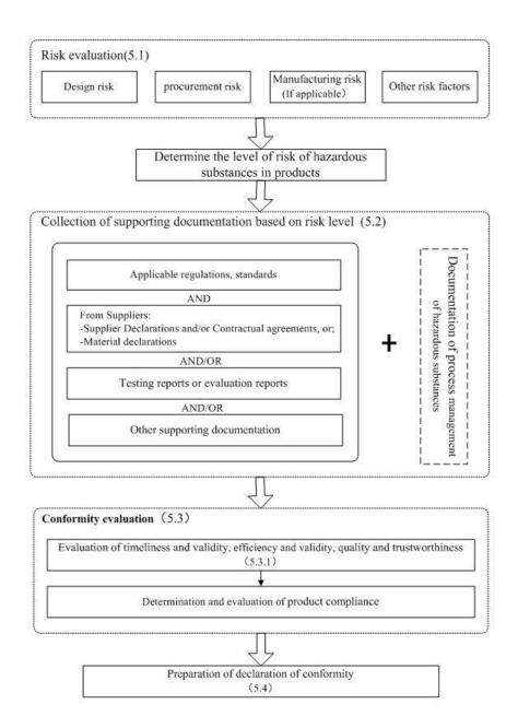
Figure 1-schematic diagram of evaluation of conformity evaluation
